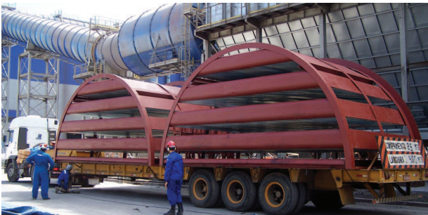
Stack Silencer for South American Power Plant
