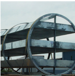
Circular Stack Inlet Silencer
